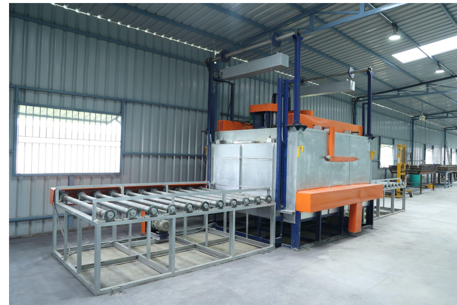
Advanced Roll-type Heating Furnace Ti Electrode Mfg Capacity: 250 m 2 p.m.
