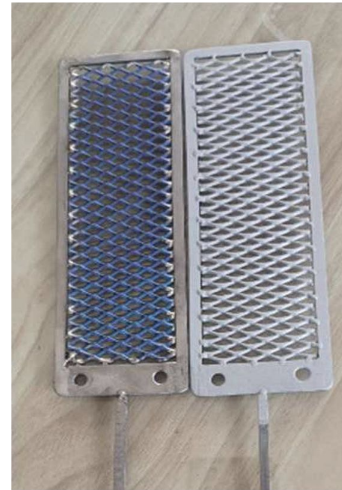
Pt Thermal Deposition
